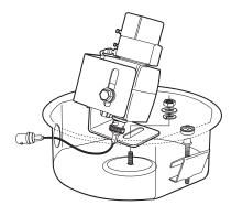
Figure 5. Installing the Camera and Lens
